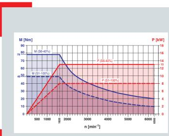
Power/Torque diagramm of the main spindle
