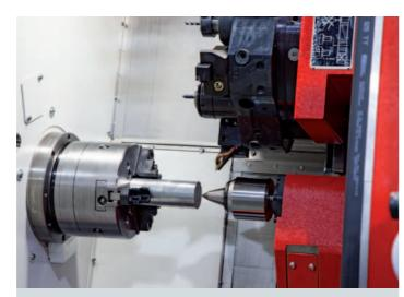
Hydraulically actuated, programmable tailstock
