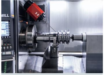
**Deep hole drilling** for diameters of up to  $6 \times 500$  mm with a maximum of 80 bar
