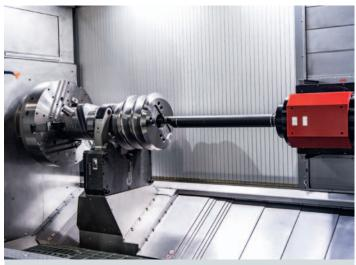
**Boring bar:** Boring bar with vibration absorption featuring a diameter of  $100 \times 100$  mm for internal turning operations. There are three specifically dimensioned tools available.
