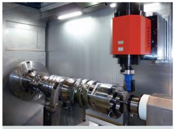
**Machining options.** From an angular tool holder to an additional U-axis – all machining processes are possible and feasible in a customised way.
