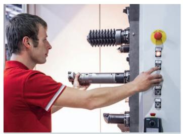
**Ergonomic loading** of the tool magazine with tools weighing up to 25 kg and measuring more than 600 mm
