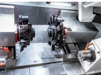
**BMT turret.** The stable BMT-55P interface replaces the standard VDI quick change system. This allows coolant pressures of up to 150 barbe implemented through the turret. Further advantages are in the accuracy and stability of the interface.
