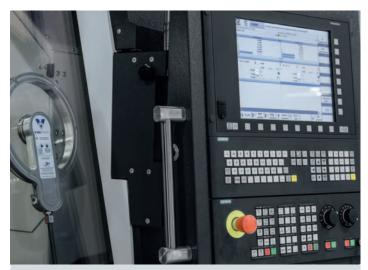
**Control.** The Sinumerik 840 D sl with operate user interface is ergonomically arranged on the right from the working area, can be swiveled 80° and changed in height by 100 mm. A side-to-side movement is standard for the 1300 versions. On the bottom is a 230 Volt socket, which can be used for any electrical device.
