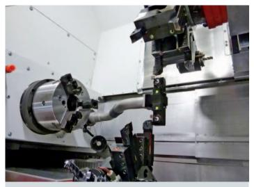
**Tool measuring.** The tool measuring arm equipped with two touch-probes enables fast and precise measuring of tools in the workspace. It is mounted manually in the bracket below the main spindle and returned to a storage tray after use.
