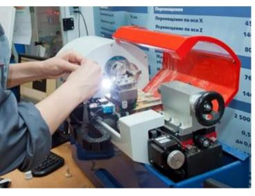
Each Junior educational machines set compris-es a machine tool, a computer with a monitor, a mouse and a keyboard, a machine control cabinet, a set of workpieces and cutting tools, and a set of training materials.
