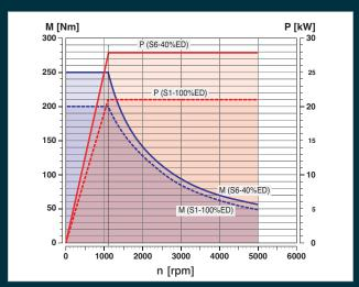
Motor characteristics for main spindle with integrated spindle motor
