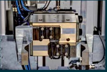
The machine is equipped with a 180° workpiece turner and a lifting station (lift height 300 mm). It can be operated pneumatically by a fixed stop or electrically by a NC axis. The gripper stroke is designed for diameters up to 220 mm. The turning station has a pneumatic drive.
