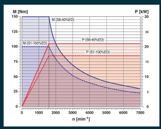
Motor characteristics for main spindle
