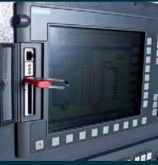
The state-of-the-art 828D control contains the latest functions from the Siemens "Operate" controller interface. Based on "solution line technology", the 828D is an ideal solution for single-channel machines like the VT 400, VT 260 and the VT 160. The communication with the controller is possible via a USB or ethernet-interface or CF-card in the front of the controller.
