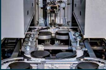
An integrated bypass line allows both simultaneous production of different workpieces, and different voltages for OP 10 and OP 20.
