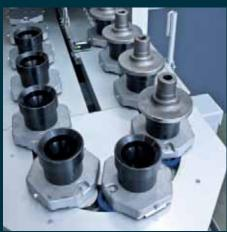
The machines can be equipped with different conveyer belts. One possibility is the standard linking system from pallet belts with spring-operated pick up stations, including 20 workpiece carriers. The feed direction is counter-clockwise. The belt is placed completely under the machines.
