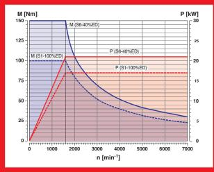
Motor characteristics for hollow spindle motor
