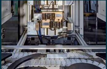
180° workpiece turner with workpiece switch for pallet 1 and pallet 2.
