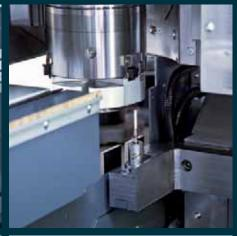
Integrated work piece measuring device: With the touch probe mounted between the work area and the loading position it is possible to gauge the work piece. During machining, the probe will be completely covered and protected from chips and coolant.
