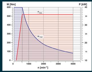
Motor characteristics for main spindle
