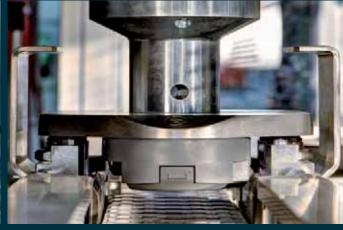
The pick-up station for the blank is designed with gimbal suspension and drive-over protection.
