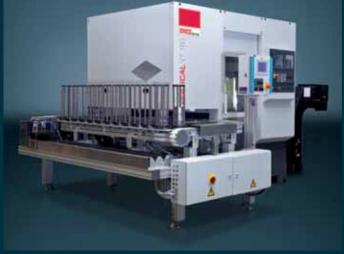
Stackable tool magazines for line production are the preferred solution for vertical machines alongside drag conveyors and pallet systems. This magazine with 10 individual stackable magazines is ideal for circular parts such as clutch plates, synchroniser rings, etc. Each magazine shaft can stack up to 60 parts, transporting 600 parts to the VT 160 vertical machine.
