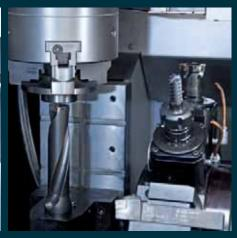
Very stable multifunctional plate. In the version without a Y axis, it also supports the use of long drilling tools.
