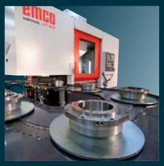
VT 400: The pallet system of the VT400 is designed to hold up to 15 parts with a diameter of 50 – 320 mm. As an alternative, a conveyor belt with carrier-prism can be offered. This can hold 12 parts with a diameter of 200 – 320 mm.
