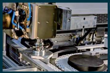
$180^{\circ}$  turning station with transport chain and workpiece carrier for the OP 20.
