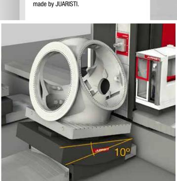
Rotary tables with capacity between 8 and 150 tonnes.
