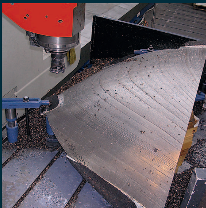
Machining of a hydraulic blade for turbines
