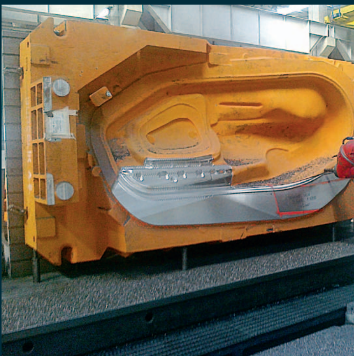
Roughing operation on a stamping die
