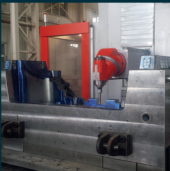
Machining through a mechanical milling head of a bumper mould
