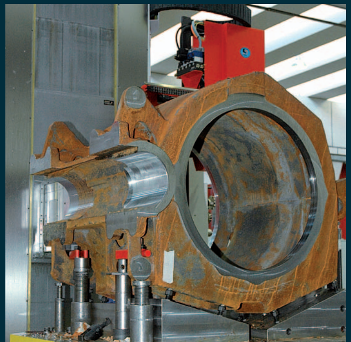
Machining of a housing of an electrical motor
