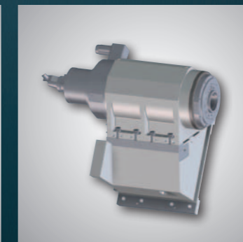
Main spindle A2-8 - Water-cooled spindle motor (ISM) - Maximum drive power: 33 kW (44.2 hp) - Maximum torque: 800 Nm (589.6 ft/lbs) - Maximum speed: 3500 rpm - Bar capacity: ø 95 mm (3.7")
