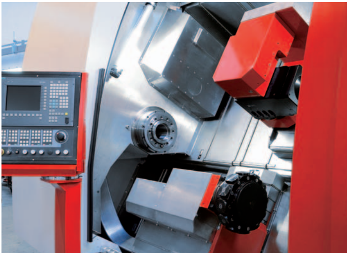
The work area provides the highest level of ergonomics with excellent accessibility to the individual components. Generous amounts of free space ensure optimal chip flow, even when machining complex materials. All guides are covered in stainless steel sheets to prevent damage.
