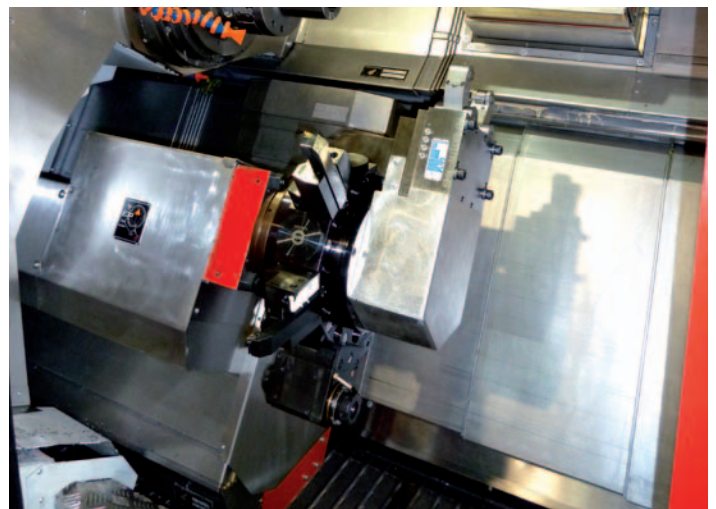
Turret steady rest: Hydraulically operated steady rest for diameter 8 – 125 mm to guarantee highest flexibility when machining shafts.
