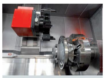
**BMT turret:** The machine's standard equipment includes one or two BMT85 12-station turrets. With a maximum of 3000 rpm, 116 Nm and 19.8 kW, this turret creates the ideal conditions for complete machining and maximum productivity. A VDI60 12-station turret is available as an option.
