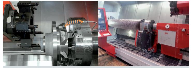
**Tailstock** / **counter spindle:** The machine is equipped with an NC-controlled tailstock (optional) with integrated bearing and MK6 quill. Workpieces with a maximum weight of 6 tons are thus supported in a safe and stable condition. With the optionally available counter spindle, it is possible to manufacture workpieces in one cycle and/or two workpieces at the same time.
