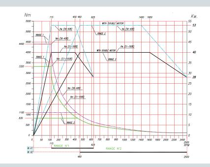
MT200 – The master/slave motor arrangement, which also serves as the C-axis, has been implemented with the EMCO spindle concept. The motors run in sync, guarantee compensation for play and make it possible to achieve the performance values and torques mentioned below (see diagrams).
