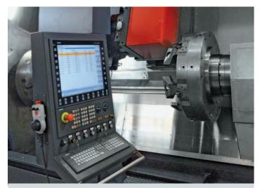
**Control system:** The machine is equipped with a Siemens 840D sl control. The scope of delivery includes a 22" display with state-of-the-art emcoNNECT control panel as well as versatile EMCO technology cycles (optional) for easy, dialogue-based programming.
