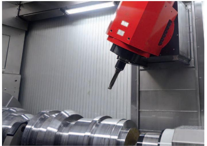
**Milling spindle.** For stable, precise and flexible drilling and milling operations. Up to 80 kW and 630 Nm of torque and 10000 rpm. Sealing air, internal HP coolant with 40 bar and externally with 14 bar and a 1400 liter paper band filter system as standard (80 bar option). The B-axis can be used at any angle or with an indexed B-axis in 2.5° steps.
