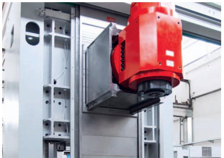
**Moving column.** Is constructed like the EMCO MECOF machines with a „Box-in-Box“ RAM structure. Thus, optimum rigidity and stability are ensured and high accuracy machining is guaranteed. The B-axis is equipped with a torque motor and integrated into the Ram design.
