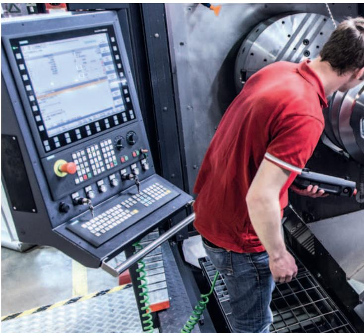
**The swivel-mounted, movable control panel** and, as an alternative, the manual control panel ensure higher flexibility and maximum access to the work area.
