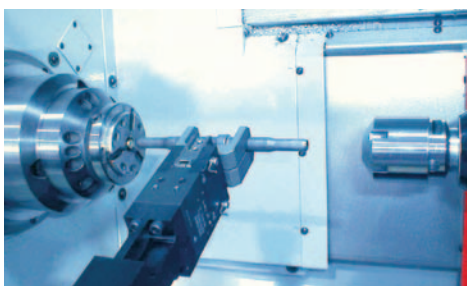
Shaft gripper for automatically loading pre-formed shafts.
