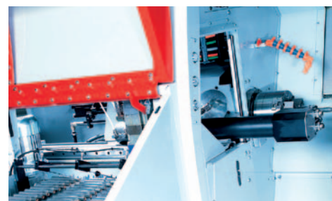
Fully automatic shaft loading. Feed-in via a conveyor belt, removal via the finished parts pick-up device
