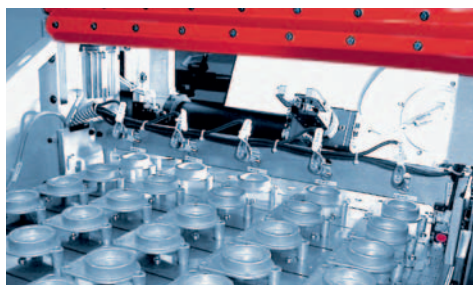
High-capacity timed conveyor system for correct directional loading of pre-formed blanks
