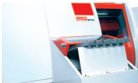
Multiple infeed chutes for loading rotationally symmetrical blanks. A sensor monitors the availability of blank parts for each infeed chute.
