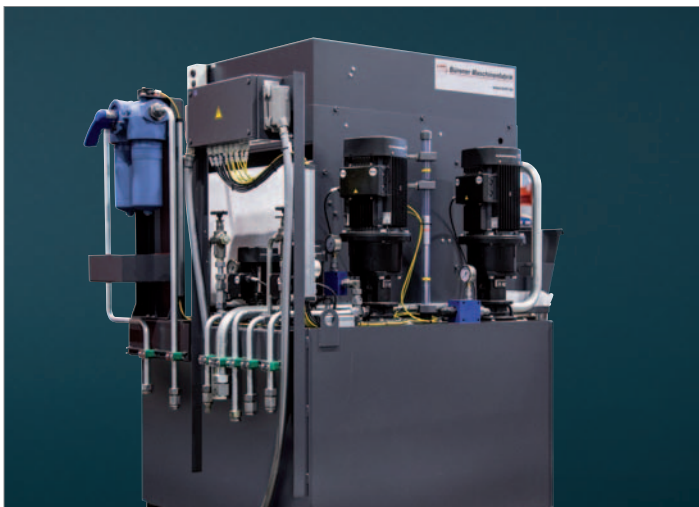
Paper-band filter system. A Paper-band filter system for coolant processing is an advantageous solution for the serial production of turned/milled parts made of aluminium, brass, steel or grey cast iron. It increases both the coolant volume and the cooling lubricant's service life. Coolant pressures of 40, 60 or 80 bar can be implemented.
