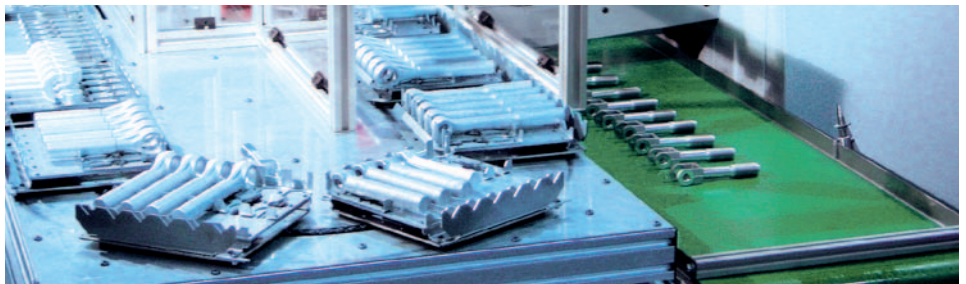
20-station pallet magazine with customer-specific pallets
