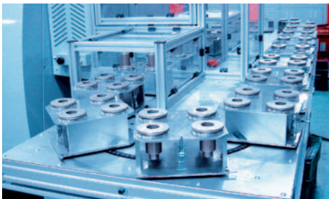
4-station pallet attachment for valve caps
