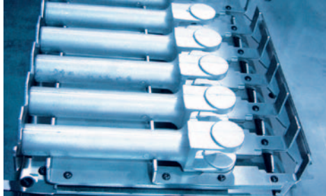
6-station pallet attachment for articulated brackets
