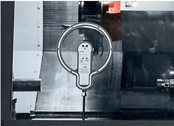
**Spin window.** The optional spin window enables the optimal insight in the working area, also during machining with coolant. Due to its very fast rotating glass plate, the coolant is slung away immediately after impact and the window stays clear.
