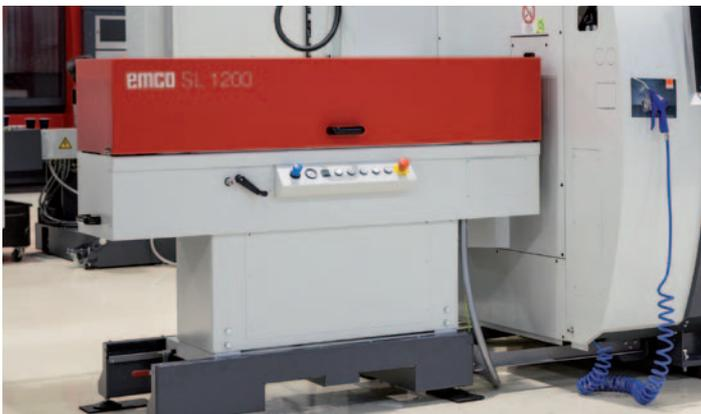
**EMCO short bar loader.** In view of the ever-increasing pressure on floorspace for machines, EMCO has developed the most compact short loader on the market: the EMCO SL1200.
