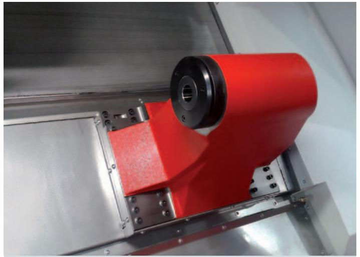
**Tailstock.** For shaft-type application, the HYPERTURN 65 offers two tailstock-versions. On the one hand an universal, hydraulic movable tailstock for manually loaded machines and on the other hand an NC-tailstock for fully automatic loaded machines. With the advantage of very short idle times.
