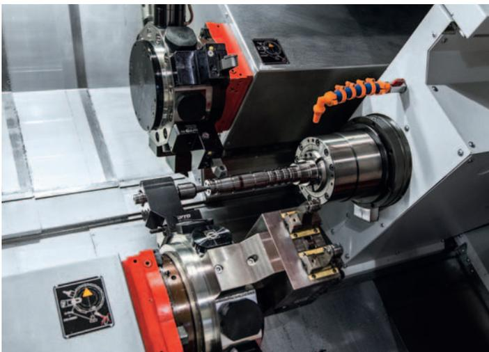
**Live-center / turret-steady-rest.** For complete machining of shaft work on the one hand in the main spindle and on the other hand in the sub-spindle, there are a live center and if needed also a turret steady rest available. So that long, slim workpieces can be manufactured precisely and without chatter marks.
