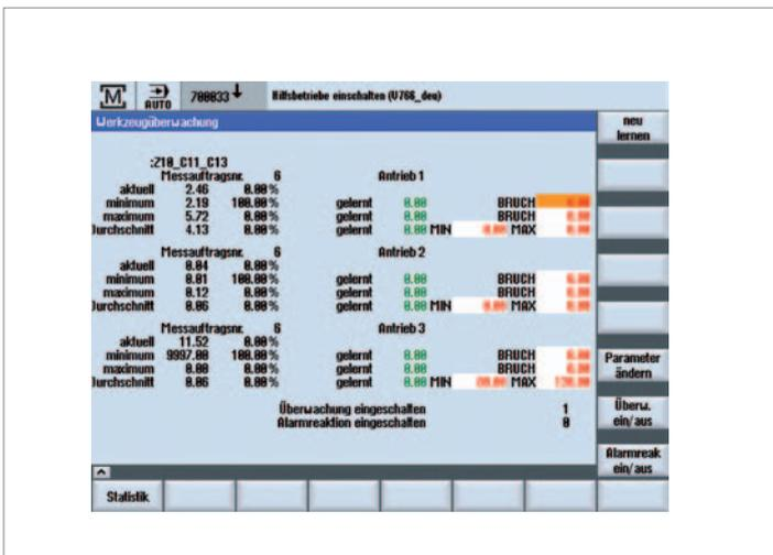
**EMCO tool monitoring system.** The tool status is monitored by evaluating the load on the various axis drive motors. Excessive loads point to tool wear or breakage. Too low a load indicates a tool is missing.
