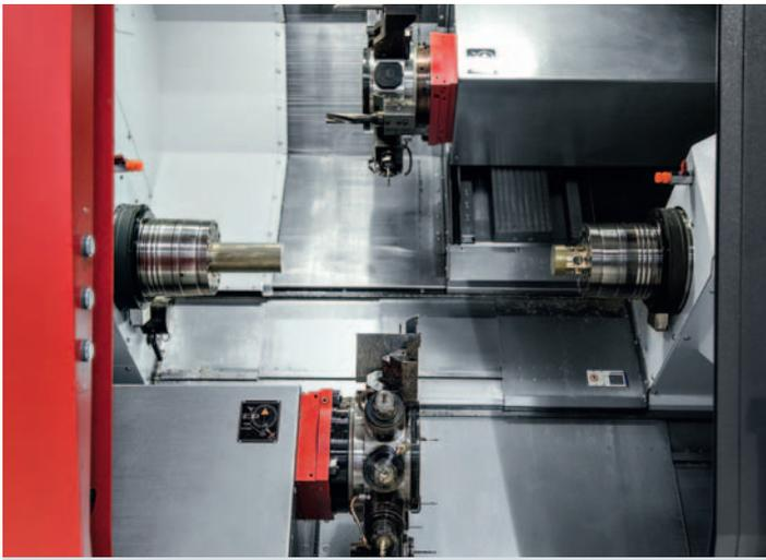
**Tool turret.** Fast 12-station servo turret with very short switching times for standardized VDI30 or VDI40 tools. All stations can hold driven tools for drilling, milling, and tapping. The operator is able to control the indexing speed with the override switch at any time.
