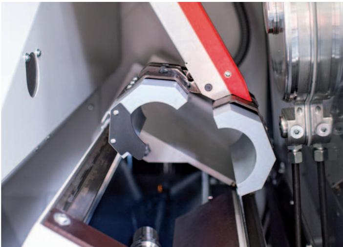
**Parts catcher.** The HYPERTURN 65's electro-pneumatic parts catcher is controlled using M functions. When needed, it traverses to the front of the work area and pivots to the spindle center. The finished part is removed from the clamping device and transferred to the catcher tray. The parts catcher then moves back to its initial position and the part is tipped onto a conveyor belt.
