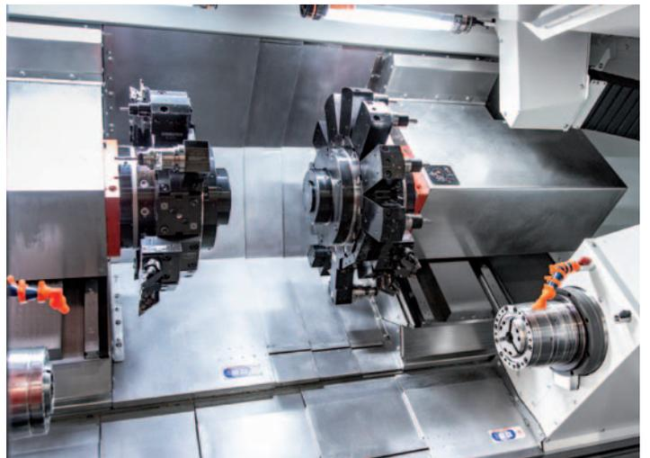
**BMT turret.** The stable BMT-55P interface replaces the standard VDI quick change system. This allows coolant pressures of up to 150 bar to be implemented through the turret. Further advantages are in the accuracy and stability of the interface.
