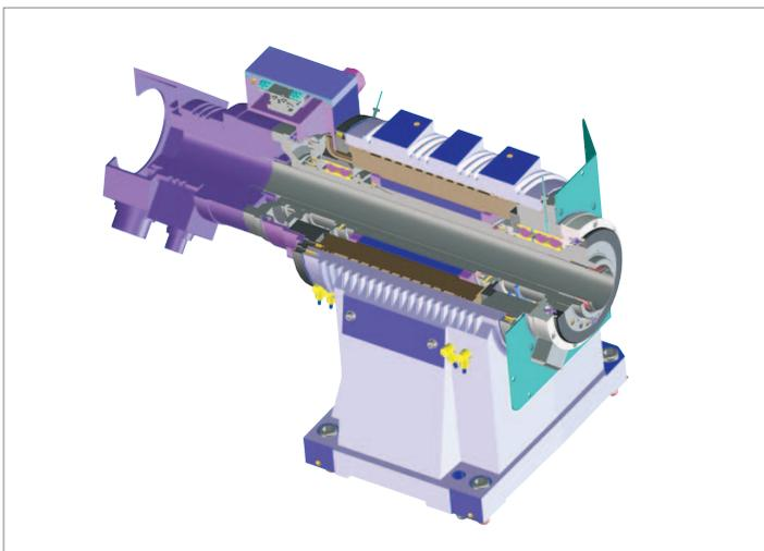
**Integrated spindle motor (ISM).** The latest synchronous technology guarantees the highest dynamics and exceptional torque in a compact design. Liquid cooling in conjunction with automatic temperature control maintains a constant temperature for all spindle motors.
