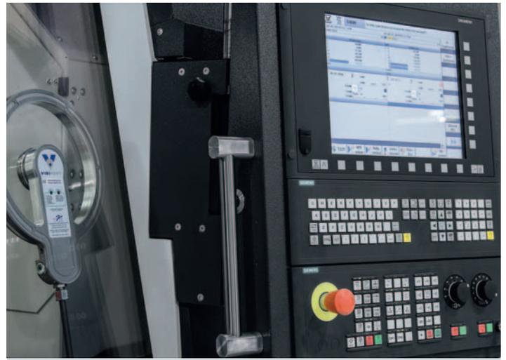
**Control.** The Sinumerik 840 D sl with operate user interface is ergonomically arranged on the right from the working area, can be swiveled 80° and changed in height by 100 mm. A side-to-side movement is standard for the 1300 versions. On the bottom is a 230 Volt socket, which can be used for any electrical device.
