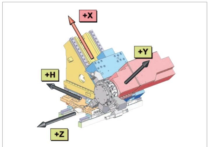
**High-precision Y-axis.** The HYPERTURN's Y-axis is designed to distribute the cutting forces over two guide planes. The result: outstanding rigidity for all turning and milling operations. The +/- 50 mm travel permits off-center milling and drilling.
