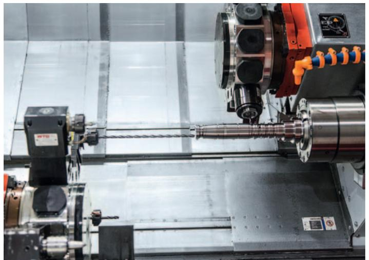
**Deep hole drilling.** For the processing of deep holes, high pressure cooling installations up to 80 / 150 bar with filtration and coolant temperature control are available. Internal coolant supply with stationary but also driven tool heads ensure a save cutting process.
