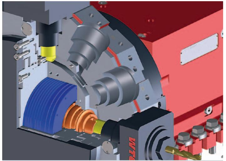
**BMT-turret.** For economical production of complex turned/milled parts with mainly milling share, there is optional the BMT-turret with water cooled direct drive. With max. 12000 rpm, 30 Nm and 10 kW, this turret offers optimal prerequisites for the complete machining.
