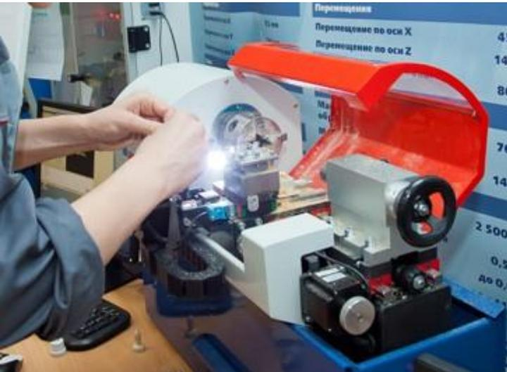
Each Junior educational machines set comprises a machine tool, a computer with a monitor, a mouse and a keyboard, a machine control cabinet, a set of workpieces and cutting tools, and a set of training materials.
