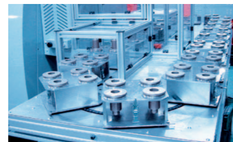
4-station pallet attachment for valve caps
