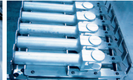
6-station pallet attachment for articulated brackets
