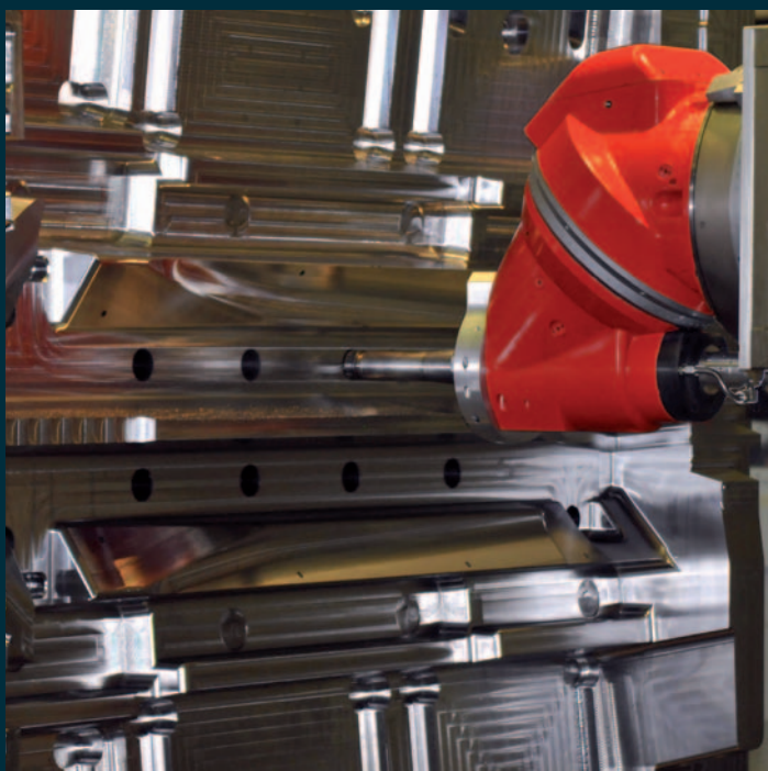
Drilling on a bumper mould by means of universal milling head (Mould & die)
