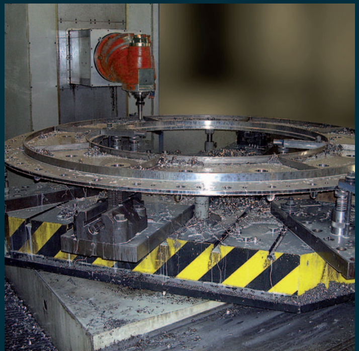
Machining of a food industry component on rotary table (Precision engineering)
