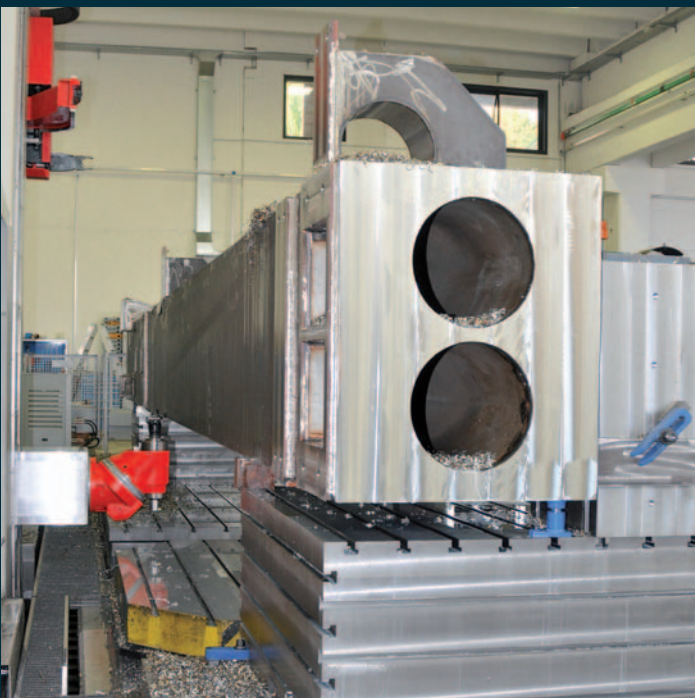
Machining of a large structure for the paper industry (Precision engineering)
