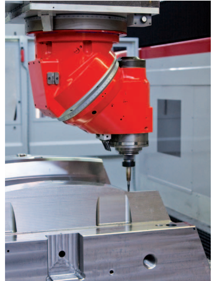
High speed machining of injection mould for bumpers in automotive industry
