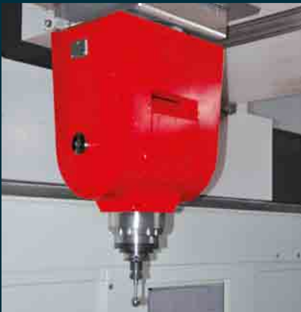
Full 5 axes fork type milling head with high-speed spindle
