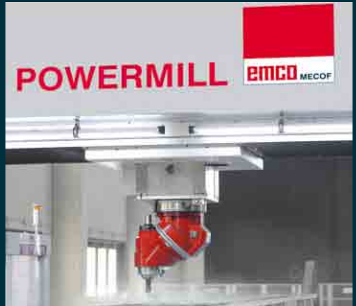
Drilling and tapping through the universal milling head on a general engineering component
