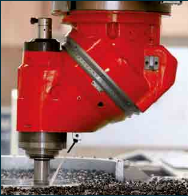
Universal milling head with automatic millesimal positioning with air/oil lubrication and water cooling
