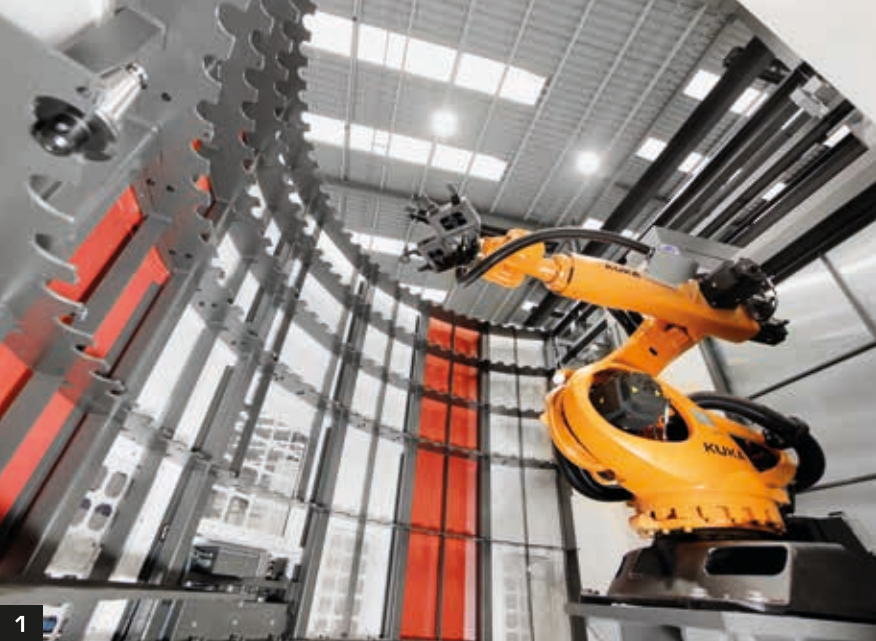
1. Robot type ATC tool changer. 2 and 3. Matrix tool changer.
