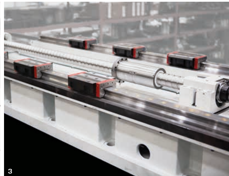
1. Thermo-symmetrical design with central head to ensure stability. 2. 4-guide column head and hydrostatic table rotation with preloaded double pinion. 3. High-precision guided LM with roller skids. 4. Integral fairing with fog extraction system. 5. Comprehensive chip and coolant collection.
