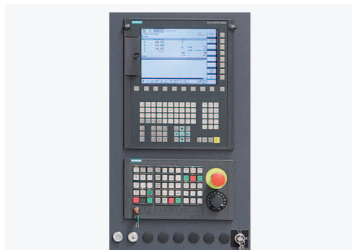
The control is built into the machine casing to keep the machine's outer dimensions as small as possible.
