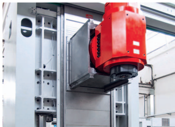
Moving column. Is constructed like the EMCO MECOF machines with a „Box-in-Box“ RAM structure. Thus, optimum rigidity and stability are ensured and high accuracy machining is guaranteed. The B-axis is equipped with a torque motor and integrated into the Ram design.
