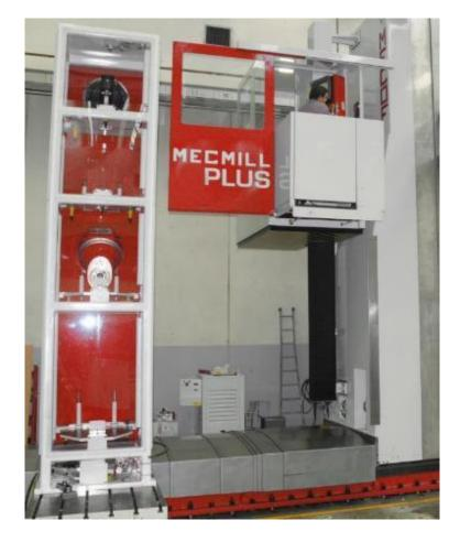
This option configuration reduces the X-axis travel of 1000 mm.
