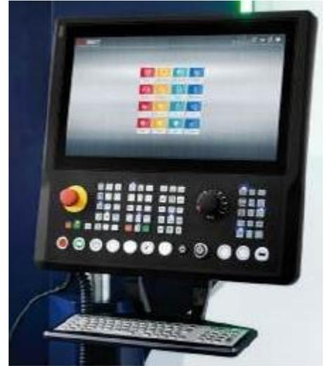
*The control hardware for emcoCONNECT consists in a 22" Panel Industrial PC (IPC427: Intel Core i3-6102E / 3x Gigabit Ethernet (IE / PN) / 4GB Memory and HMI Operating System Windows 10 IoT Enterprise Ultimate / 180GB Solid-State Drive SATA) and a customized Premium PC keyboard and machine control panel.*
