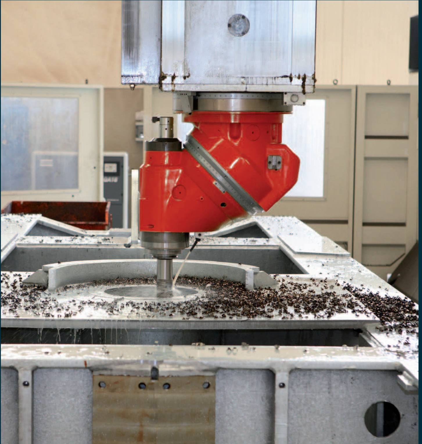
Mechanical machining of a cableway frame
