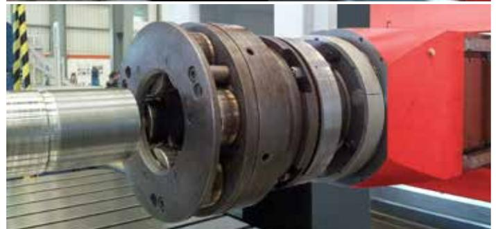
**MX7 RAM** Turbine rotor slot machining with large mill disc
