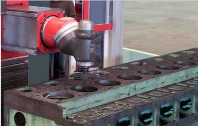
**MX7 RAM** Engine block milling and boring
