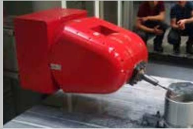
**AK2 Twist head 2-axes continuous rotation**
