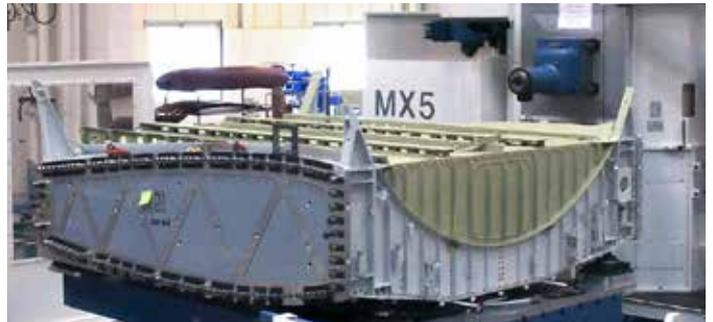
**MX5** Aircraft central fuselage on rotary table
