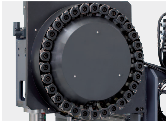
Tool magazine. Is equipped with 30 tool stations. At the version with 24.000 U/min the spindle has a HSK-A40 recording.
