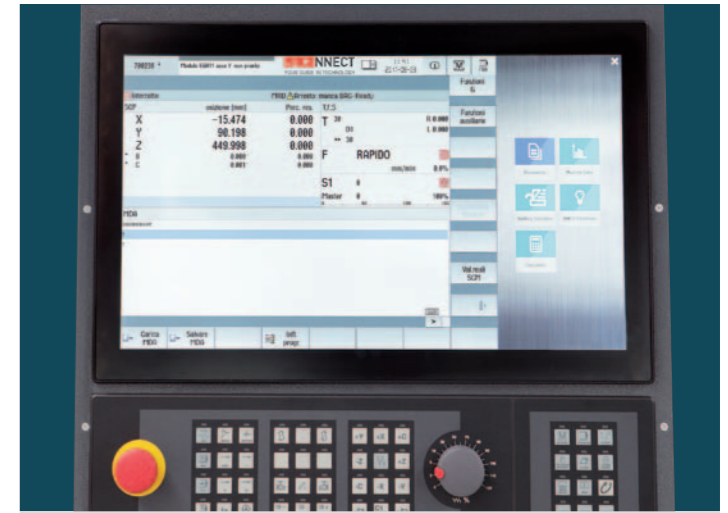
Sinumerik 840D sl incl. Shopmill. Sinumerik 840D sl incl. Shopmill: The Sinumerik 840D sl incl. Shopmill is a universal and flexible CNC system and offers free contour programming, Moving cycles for complex contours, fast reference point setting with touch probe systems, tilting the working plane, Cylindrical surface machining, 3-D tool compensation, fast execution through short block processing times.
