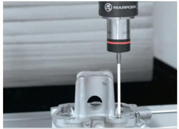
**Measurement systems.** Tools measurements to reduce setup times during tool changes, as well as work piece measurements to verify dimensions or to find zero locations. The work piece measurement is radio.
