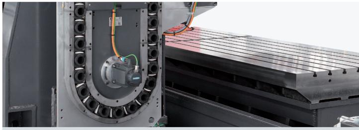
**Tool magazine:** available with steady tool magazine on 3-, 4- or 5-axis version, or with moving chain magazine on 4- and 5-axis version. Tool change on steady magazines with dual arm grippers at the X-axis limit, with 40 tool stations (optional 80). Tool change on the moving magazine (40 as standard, 60/120 as option) fast and safe, all along the X-axis and at the extreme limit of the Z- and Y-axis. An external tool changer "tower" is available upon request.
