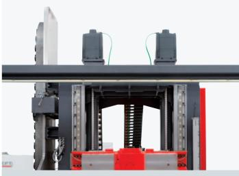
**Z-axis travel:** In order to attain precision Z-axis rapid travel at speeds of 40 m/min, and due to its large mass, this axis is powered by two ball screw drives and two motors in a master-slave configuration.
