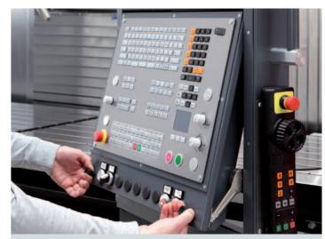
**Control unit:** The operator panel can travel, rotate and be adjusted in the direction of the work space. This ergonomic design provides ideal working conditions for the operator.
