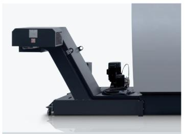
**Hinge type conveyer:** The chip rinsing system washes chips into the hinge type conveyer, which then automatically transports the chips from the machine into the customer provided container.
