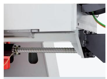
**Y-axis:** The Y-axis has a ram configuration. This design uses long way guides in order to attain the required rigidity. Its high precision is guaranteed by the motor installed direct drive on the screw.
