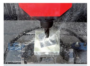
**Coolant through the spindle.** The spindle can be optionally flooded with high-pressure coolant (25 to 60 bar [362,59 to 870,23 psi]). This ensures reliable chip removal from holes and pockets and reduces cycle times for this type of machining.
