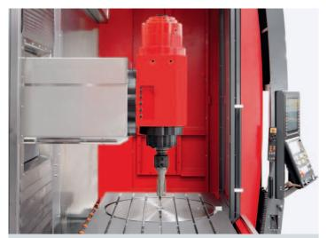
**Milling spindle:** The machine is equipped with a liquid cooled motor spindle with compelling performance specs. At spindle speeds of 15000 rpms, a power rating of 46 kW, and a torque of 170 Nm, the machine is also suited for heavy-duty machining. A motor spindle 18000 rpm is available with HSK A63.
