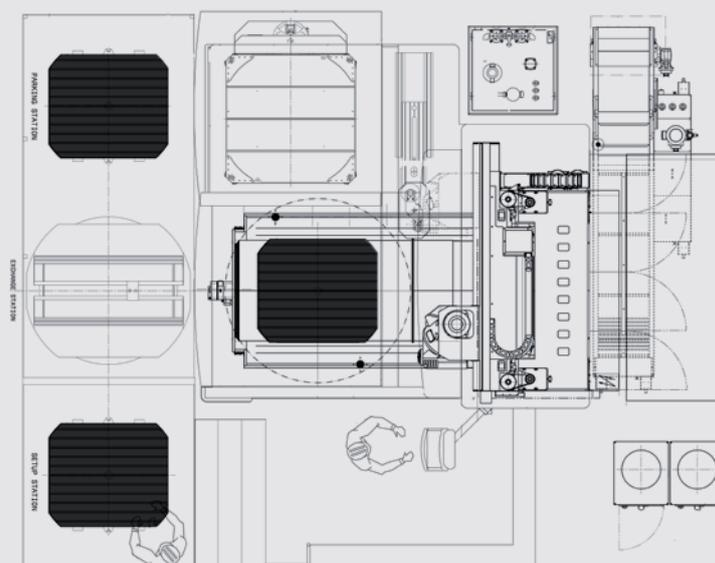
**Productivity optimisation.** Automatic pallet exchange systems improve the machinery's productivity and reduce the idle time, which is mainly due to the fixturing of the workpiece. The Umill 1500 and Umill 1800 configurations offer several solutions to meet the requirements of each single customer. Our pallet exchange systems offer the best compromise between greater load capacity and smaller overall dimensions in the workshop, whilst ensuring shortest possible pallet exchange times.
