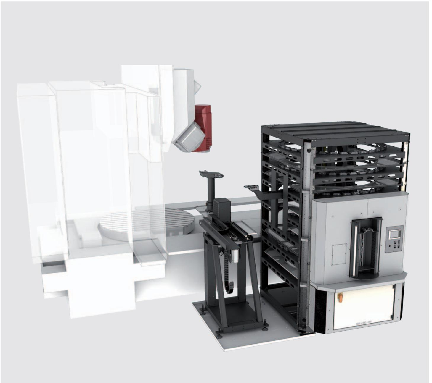
**Placed outside the work space and separated from the machine base.**
