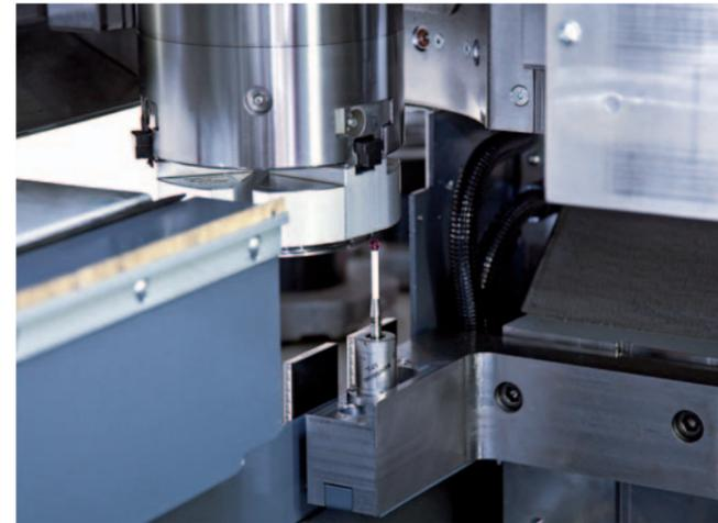
Integrated work piece measuring device: With the touch probe mounted between the work area and the loading position it is possible to gauge the work piece. During machining, the probe will be completely covered and protected from chips and coolant.
