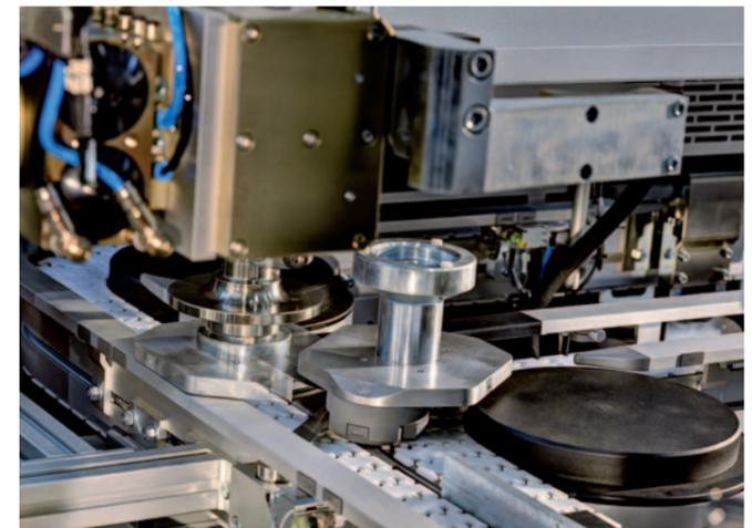
180° turning station, turning process completed: Workpiece carrier for the OP 10 without a workpiece moves back via a switch for loading with blanks. Workpiece carrier for the OP 20 with workpiece moves to processing of the second operation.
