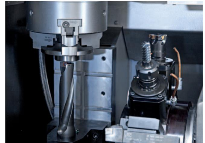
Very stable multifunctional plate. In the version without a Y axis, it also supports the use of long drilling tools.
