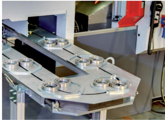
VT 160 with two track loading. Two track loading is possible up to a part diameter of 100 mm. The benefits for you: good parts supply, short chip-to-chip times up to 5.5 seconds.
