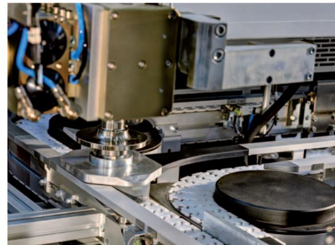
180° turning station with transport chain and workpiece carrier for the OP 20.
