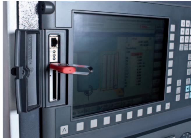
The state-of-the-art 828D control contains the latest functions from the Siemens „Operate“ controller interface. Based on „solution line technology“, the 828D is an ideal solution for single-channel machines like the VT 400, VT 260 and the VT 160. The communication with the controller is possible via a USB or ethernet-interface or CF-card in the front of the controller.
