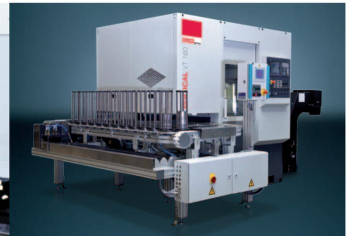
Stackable tool magazines for line production are the preferred solution for vertical machines alongside drag conveyors and pallet systems. This magazine with 10 individual stackable magazines is ideal for circular parts such as clutch plates, synchroniser rings, etc. Each magazine shaft can stack up to 60 parts, transporting 600 parts to the VT 160 vertical machine.
