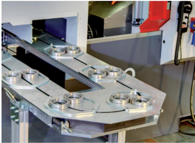
VT 260 with two track loading. Two track loading is possible up to a part diameter of 100 mm.
