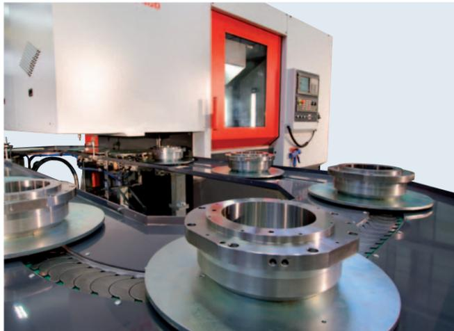
The pallet system of the VT400 is designed to hold up to 15 parts with a diameter of 50 – 320 mm. As an alternative, a conveyor belt with carrier-prism can be offered. This can hold 12 parts with a diameter of 200 – 320 mm.
