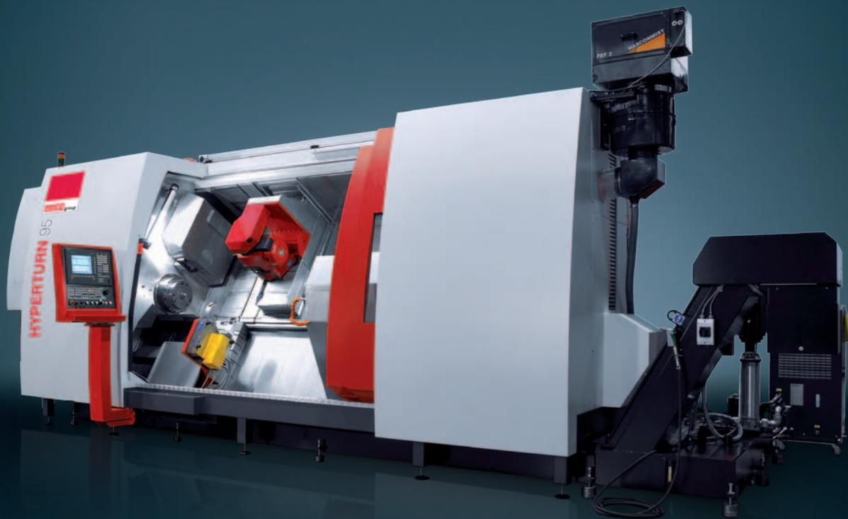
For complex, complete machining, the system uses a modular, building block system with two base lengths (1700 or 2300 mm), two spindle sizes, with a milling spindle and a B-axis or with two turrets.
