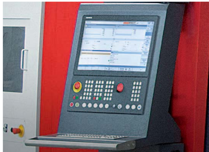
emcoCONNECT's hardware basis is a 22" industrial touch control panel combined with an industrial PC (IPC).
