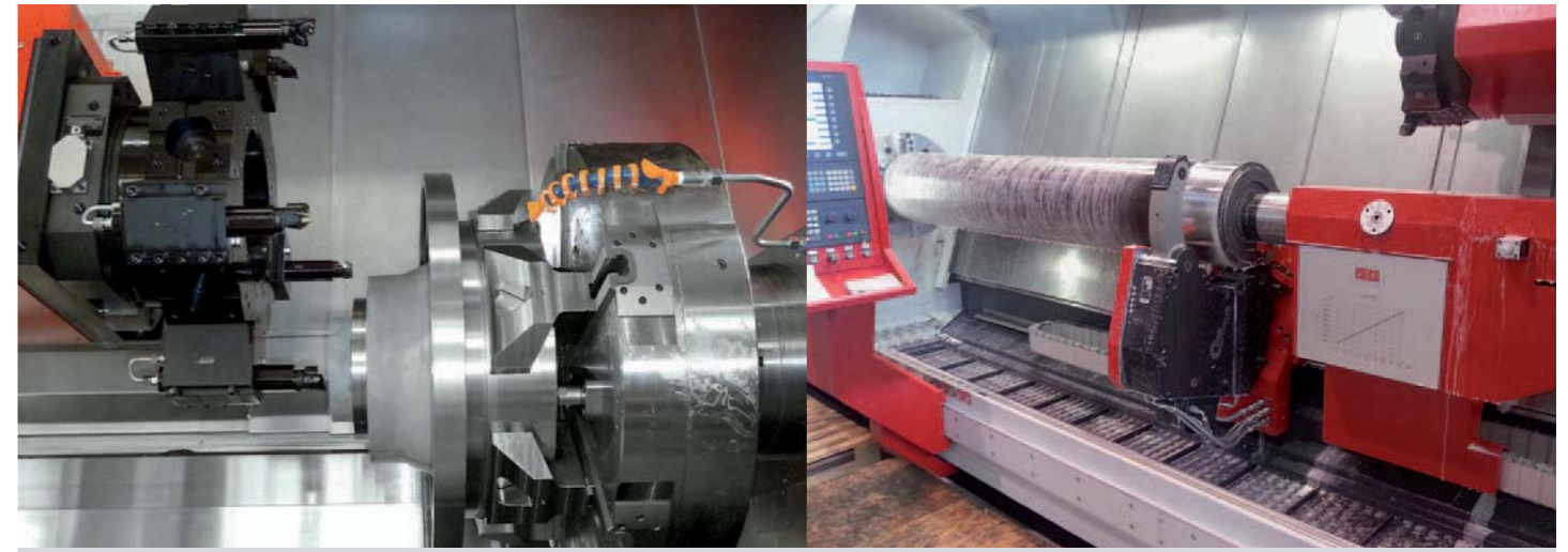
Tailstock / counter spindle: The machine is equipped with an NC-controlled tailstock (optional) with integrated bearing and MK6 quill. Workpieces with a maximum weight of 6 tons are thus supported in a safe and stable condition. With the optionally available counter spindle, it is possible to manufacture workpieces in one cycle and/or two workpieces at the same time.
