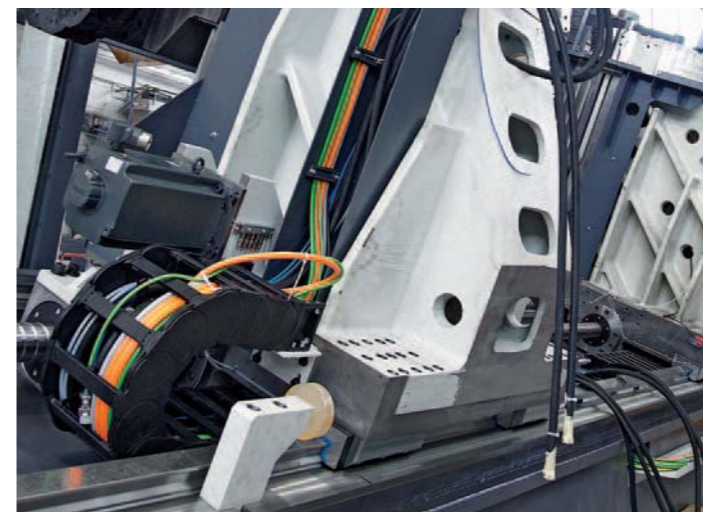
High-precision Y-axes: The Maxxturn machine concept has been designed in such a way that the Y-axis is fitted at an angle of 90°. Due to large, widely spaced and prestressed linear roller guide rails, this Y-axis ensures optimum machining results with maximum stability and short projection lengths (possible for up to two turrets).
