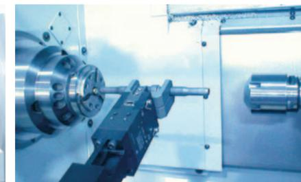
Shaft gripper for automatically loading pre-formed shafts.
