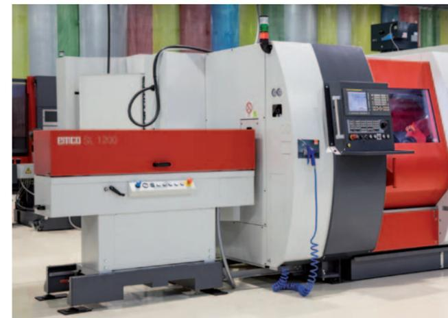
**EMCO SL1200.** Space-saving and cost-effective bar loading magazine. Operation and programming could not be easier. May also be used for loading single items through the lathe's main spindle.
