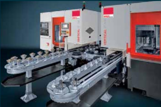
The DUO VT is available as a meander design, which is equipped with a 180° turner and an optional switch. Up to 25 pallets can be used per operation. Separate controls exist for different operating modes (manual, setup, automatic).
