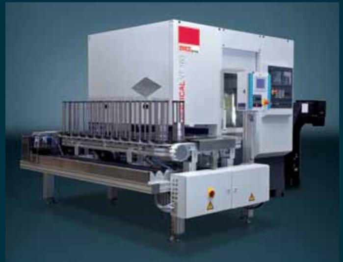
Stackable tool magazines for line production are the preferred solution for vertical machines alongside drag conveyors and pallet systems. This magazine with 10 individual stackable magazines is ideal for circular parts such as clutch plates, synchroniser rings, etc. Each magazine shaft can stack up to 60 parts, transporting 600 parts to the VT 160 vertical machine.
