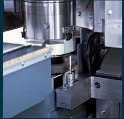
Integrated work piece measuring device: With the touch probe mounted between the work area and the loading position it is possible to gauge the work piece. During machining, the probe will be completely covered and protected from chips and coolant.
