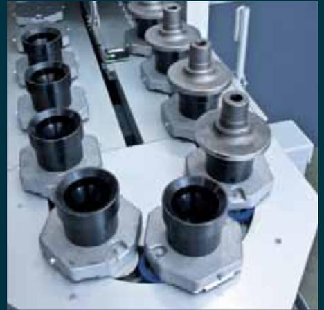
The machines can be equipped with different conveyer belts. One possibility is the standard linking system from pallet belts with spring-operated pick up stations, including 20 workpiece carriers. The feed direction is counter-clockwise. The belt is placed completely under the machines.
