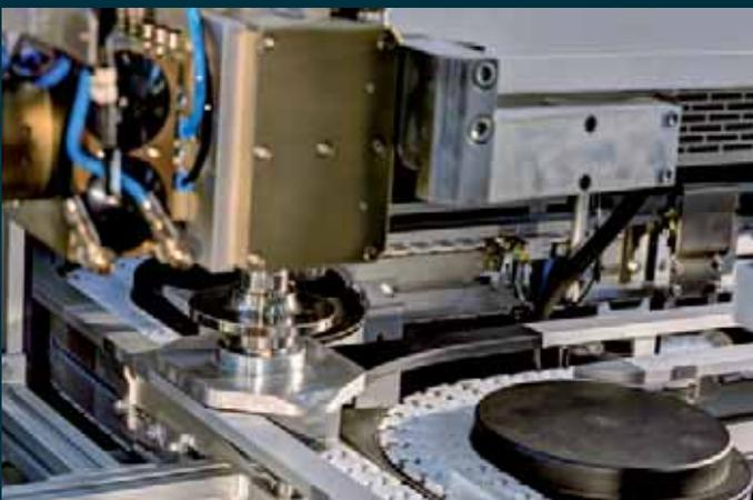
180° turning station with transport chain and workpiece carrier for the OP 20.
