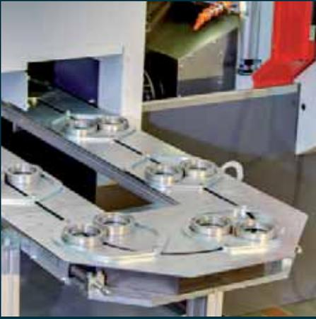
VT 160 with two track loading. Two track loading is possible up to a part diameter of 100 mm.
