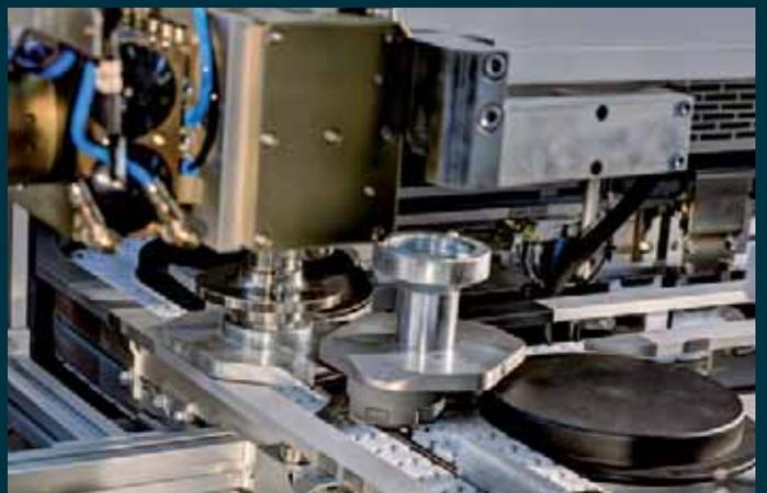
180° turning station, turning process completed:
