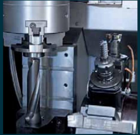
Very stable multifunctional plate. In the version without a Y axis, it also supports the use of long drilling tools.
